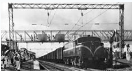
This is one of the DC 3,000 V 3,600 HP electric locomotives that enjoyed extensive service in India. Two years later, Hitachi followed up by delivering the first of seven DC 1,500 V 4,050 HP electric locomotives.
