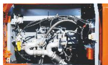
Grouped remote filters and inspection points
