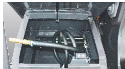
Electric fuel refilling pump
