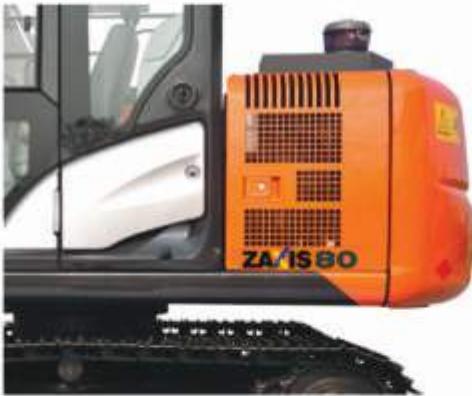
Covers with higher cooling efficiency
