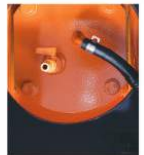
Drain cock & cleaning port
