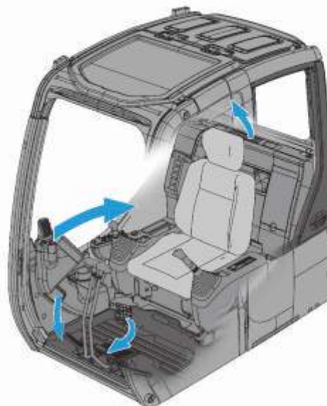
Full-auto air conditioner air outlets
