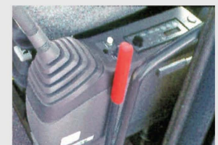
Pilot-control shutoff lever
