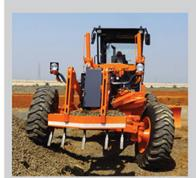
Built from high strength structural steel with Oscillation about the central axle mounting pin.
