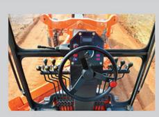
TG160 offers both manual and automatic speed selection to maximize operator efficiency both in rough and fine grading jobs.
