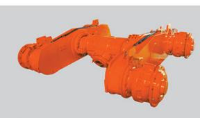
ZF make Tandem axle has high strength structural steel construction. Oscillation of Tandem each way is 18<sup>0</sup> 100 % differential lock helps reduce tyre wear.
