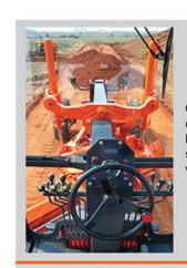
Good and wide visibility offers clear view of the mold board heel. The elevated operators seat helps in good rear visibility.
