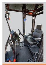
Ergonomically designed cabin with three way adjustment of operator seat, adjustable steering wheel and steering column for high operator comfort.
