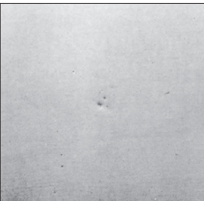
Pinhole texture by inappropriate rust proof.
